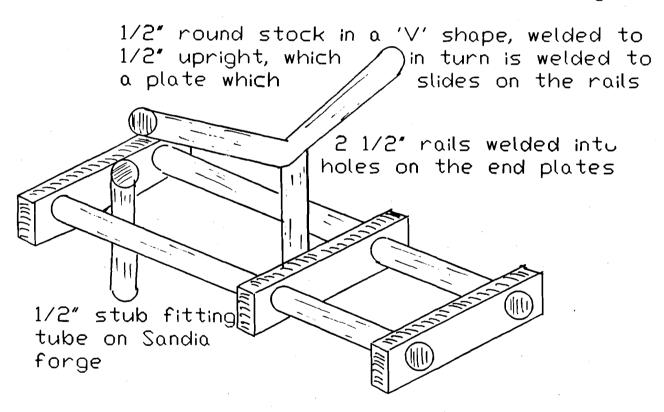
End plates and mobile plate made with  $1/2" \times 1" \times 3"$  stock, with 2 1/2" holes drilled 2" apart. Holes in mobile plate reamed slightly over 1/2".
